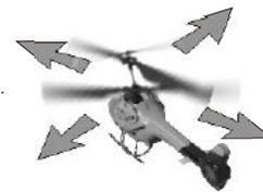
Only slight inputs are needed to move the helicopter. Too much input can cause the helicopter to tip too far to one side. Continue to make small corrections to keep it level.
