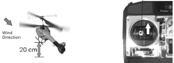
Keep focus on the nose of the helicopter and correct using the rudder control any time the nose turns too far left or right.
