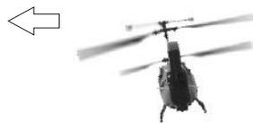
Helicopter tilts/drifts left by adding left Aileron input.
