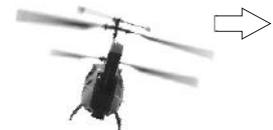
Helicopter tilts/drifts right by adding right Aileron
