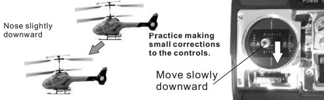
When landing, dip the nose downward slightly to avoid having a tail rotor strike. Landing with the tail drooping may allow the tail blades to touch the ground which will break them.
