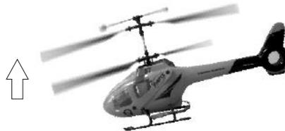
Helicopter tilts/drifts forward by adding upward Elevator input.
