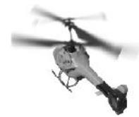
The higher the helicopter flies the more corrections you will need to make to control it. Make note of any tendency to drift in order to make corrections to trims or pushrods (page 5, section 7).
