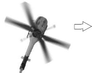
Helicopter nose moves right by decreasing the tail motor speed.
